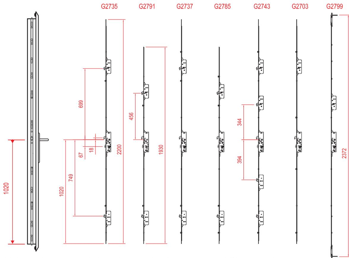
**All door locks are twin spindle and accept shootbolts as standard (Dimensions in mm).**
